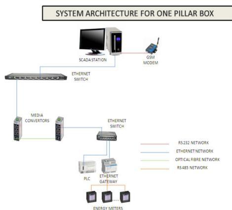
**Fig. 2.** System architecture for Pillar Box.
