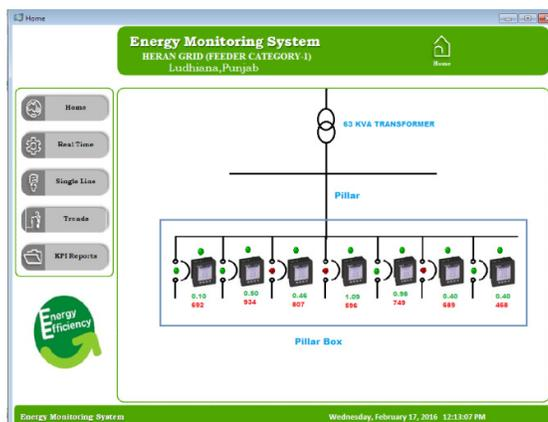
Fig. 3. Single Line Diagram of Transformer.
