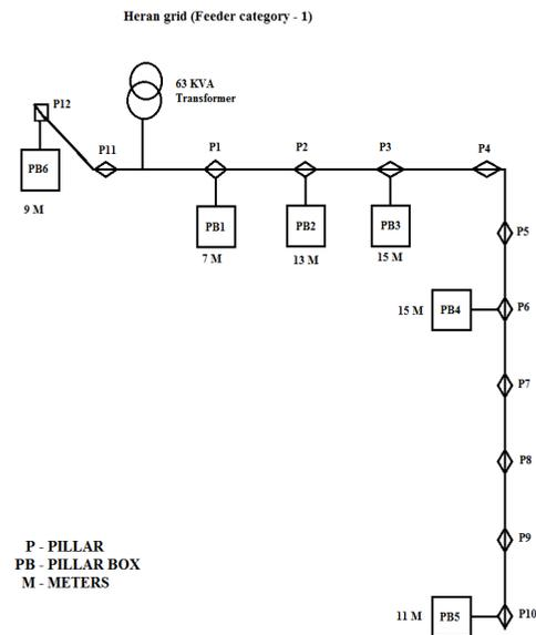
**Fig. 1.** Single Line Diagram Of 63 KVA Transformer.
