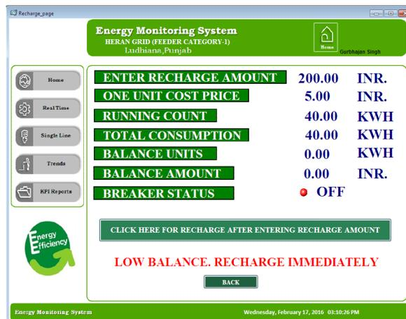
Fig. 9. Breaker Status when balance is Zero.
